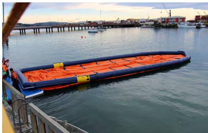
FIGURE 1: NORTHLAND REGIONAL COUNCIL'S FAB DOCK IN USE. ENVIRONMENT SOUTHLAND'S FAB DOCK WILL BE SLIGHTLY LARGER TO ACCOMMODATE THE AVERAGE VESSEL THAT TRAVELS TO THE FIORDLAND MARINE AREA
