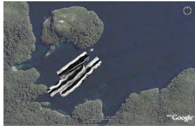
Figure 1. Side-scan sonar tracks, each 60 m wide
