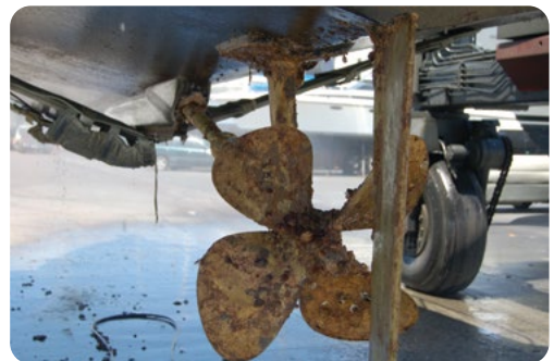
Biofouling on vessel propeller. MPI
