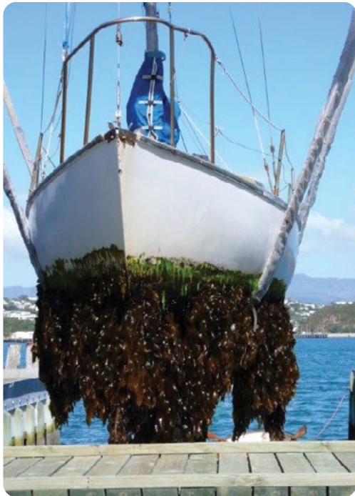
Undaria pinnatifida biofouling on vessel hull. MPI
