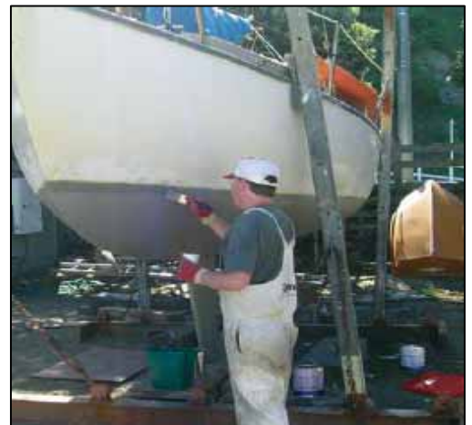
Applying of antifoul paint to prevent marine growth.
