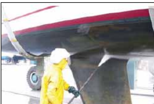
Keeping a boat hull clean with a quick waterblast.
