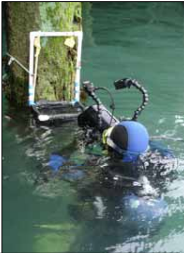
A NIWA staff member checking the marine growth on a wharf pile. Photograph supplied by NIWA.
